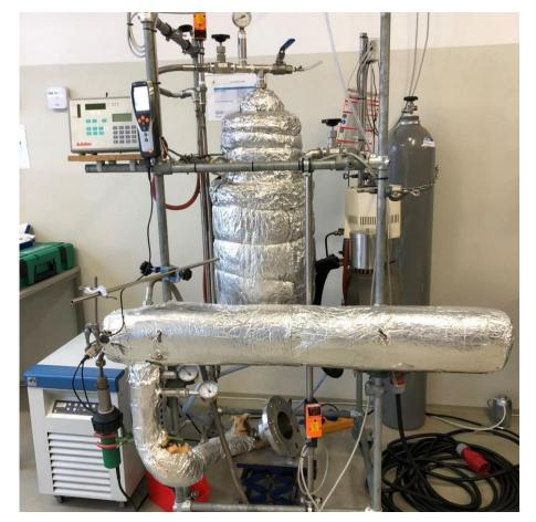
Pilot plant for  $\rm CO_2$  capture and storage in ttz Bremerhaven
